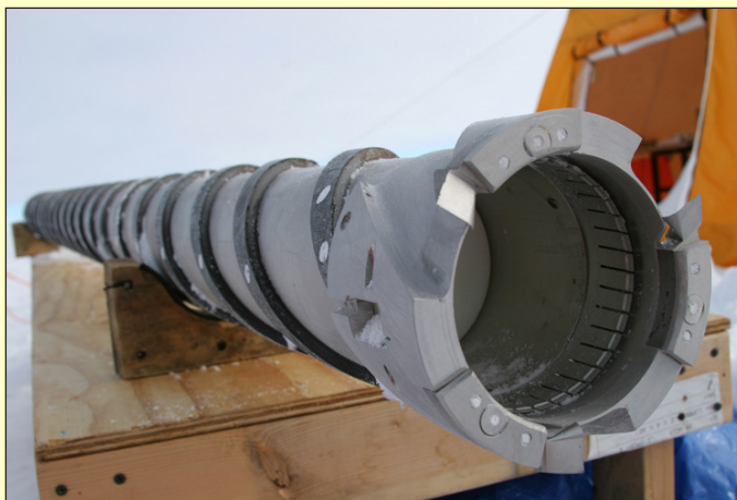
A drill used to extract ice cores in Antarctica. Ice drilling is vital to a wide range of scientific research. The IDPO/IDDO will work with the U.S. ice science and drilling communities to facilitate planning efforts and be proactive in the planning and coordination that is necessary to form and execute continuously evolving ice drilling and science programs.
